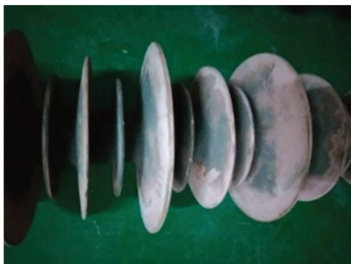
图 1 500 kV 高压输电线路退役绝缘子串 Fig. 1 Composite insulator string retired from 500 kV AC transmission line
