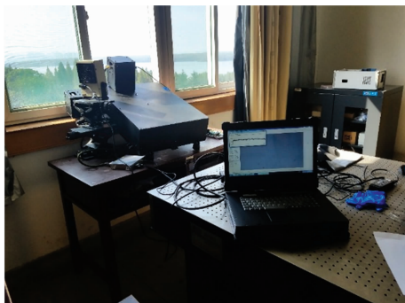
图 4 中高层大气 OH 自由基超光谱探测仪大气散射观测实验 Fig. 4 Scattered radiation observation by hyper-resolution spectrometer for mesospheric OH radical
